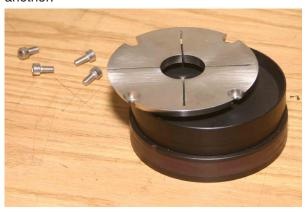
1.3 Loosely insert 4 M5 screws in the notches of the clamp into the shaft adapter face. Do not tighten at this time. The wheel is ready to install.
