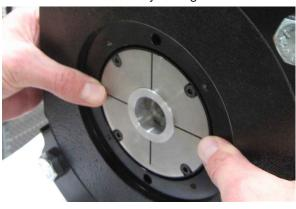
2.6 Tighten Shaft Clamp's 4, M5X.0.7M Screws in a star pattern (~35 in-lbs, 90in-lbs max) to engage the clamp in the correct position.
