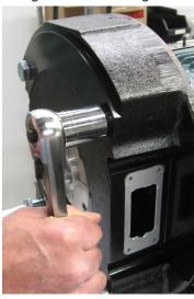
2.5 Position the Pulsewheel to its correct position under the sensor modules by sliding the shaft adapter along the shaft until the front face is flush cover surface of the housing. The clamp screws may need to be loosened to allow easy sliding.
