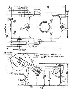
HLD-1, 2, 3 & 4 in Standard Enclosure HLD-5, 6, 7 & 8 in Dust-tight Enclosure
