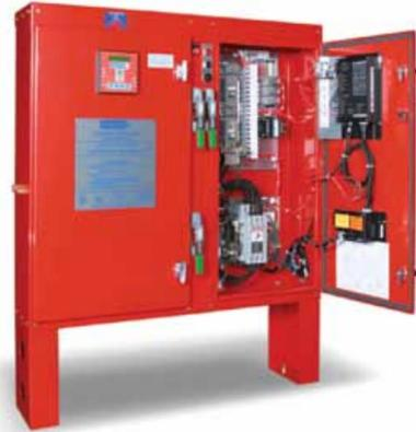
Fire Pump Controllers with Automatic Transfer Switches provide for power connections to the fire pump motor for the primary power source or an alternate emergency supply. If the primary power supply fails, an automatic transfer is made to the emergency supply. Automatic retransfer to normal power supply will occur after restoration of normal power.
