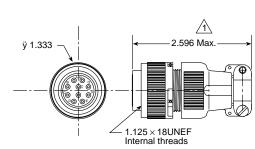
Length is with threads fully engaged.
