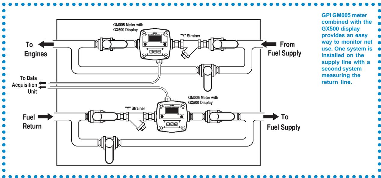
GPI GM005 meter combined with the GX500 display provides an easy way to monitor net use. One system is installed on the supply line with a second system measuring the return line.
