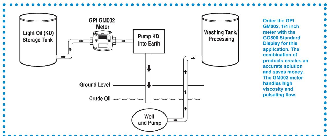
Order the GPI GM002, 1/4 inch meter with the GG500 Standard Display for this application. The combination of products creates an accurate solution and saves money. The GM002 meter handles high viscosity and pulsating flow.
