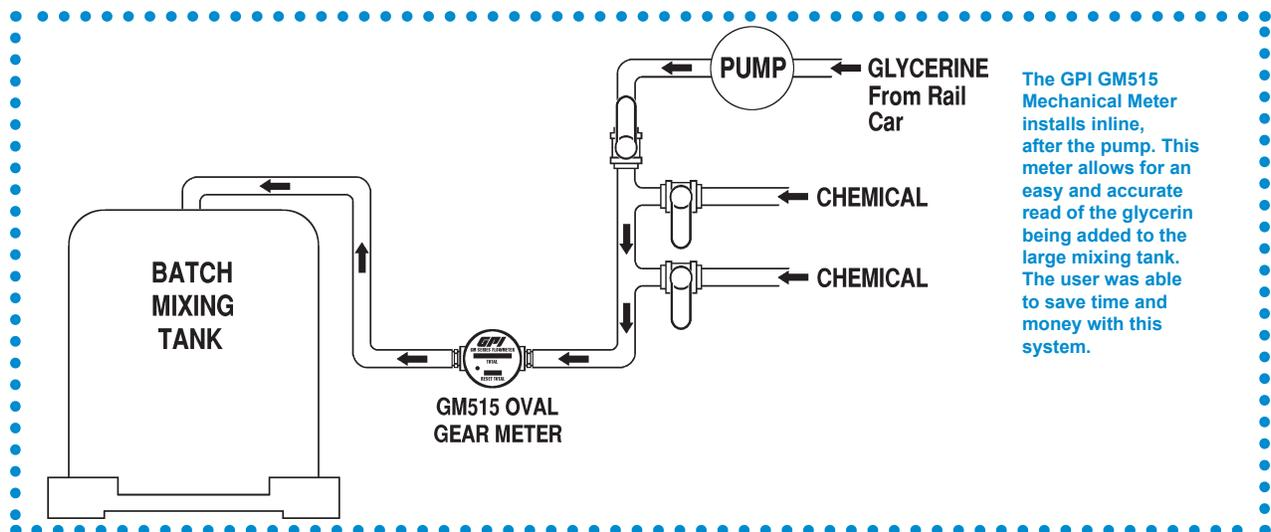
The GPI GM515 Mechanical Meter installs inline, after the pump. This meter allows for an easy and accurate read of the glycerin being added to the large mixing tank. The user was able to save time and money with this system.
