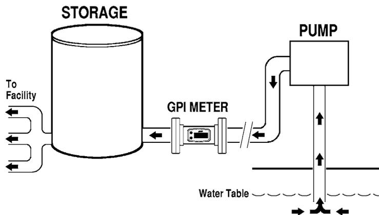
The GPI TM400-F meter fits in the line between the pump and the storage tank. The display is easy-to-read and provides rate of flow plus batch and cumulative totals. Flow Range of the TM400-F is 60 - 600 GPM (227 - 2271 LPM).
