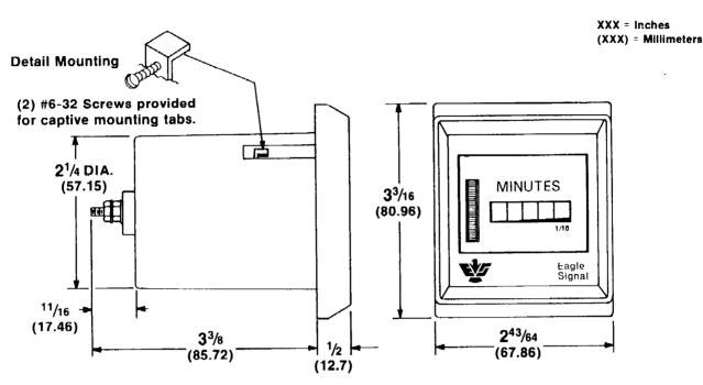
Requires 23/8 diameter panel cutout for mounting. 1/2 maximum mounting panel thickness.
