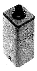
The CG900 series is a delay timer available in 19 time ranges from 0.5 seconds to 30 hours. The timer uses CMOS integrated circuits for the timing function. The desired delay time is set by the adjustment of a calibrated knob referenced to an index mark on the housing. At time out, a DPDT relay is actuated for control of output loads.
