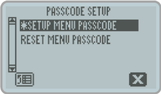
Figure 20: Asterisk indicates enabled passcode
