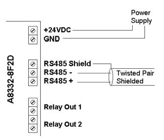
If the A8332-8F2D receives any Modbus traffic on the RS485 port, the yellow RX led should blink.
