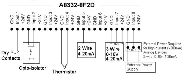
8) Power up the A8332-8F2D. The Alive LED should blink once per second. Use the AcquiSuite or the Obvius Config Console software or AcquiSuite to confirm the operation of each input.
