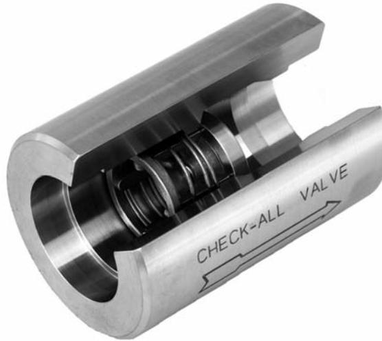
The **Universal Socket Weld (US)** check valve is a one piece body machined from bar stock with socket weld ends and is designed for a minimum pressure drop. It carries rugged, dependable Check-All trim and there are a wide variety of seat materials and cracking pressures to choose from. The socket parts are machined to ASME/ANSI B16.11 dimensions.
