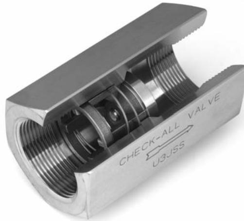
The **Universal Low Pressure (U3)** check valve is a one piece body machined from bar stock and is designed for minimum pressure drop. The valve has a light weight compact design that provides maintenance-free, dependable service. Threads are per ASME B1.20.1. Also available with ISO 7 “Rp” threads. (UR)
