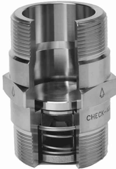
The **Connector (CN)** valve is a check valve with a pipe nipple or connector housing. It is designed to be used in installations where a check valve with male pipe threads are required. The Connector valve is adaptable for use as a check valve, vacuum breaker, or low pressure relief valve. Two valves used in combination make an excellent low pressure relief/vacuum breaker. Threads are per ASME B1.20.1. Also available with ISO 7 “R” threads (CR).
