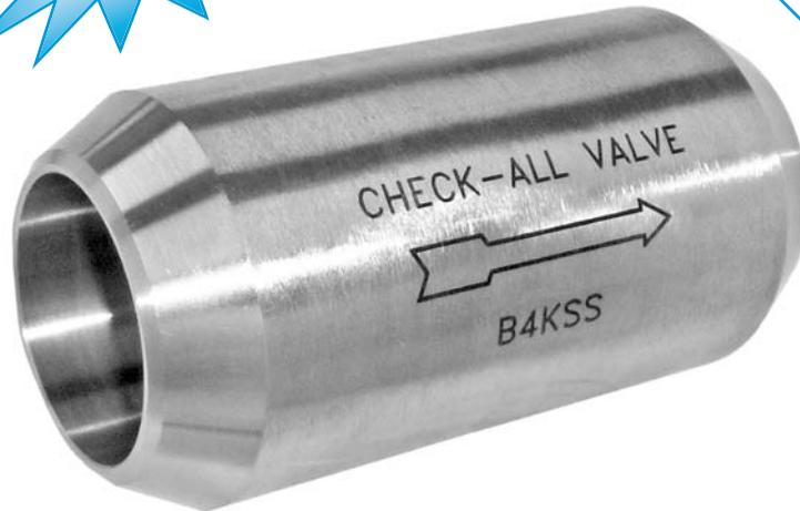
The **Butt Weld (B4)** check valve is a one piece body machined from bar stock, eliminating porosity concerns and providing uniform density for more consistent welds. Made to ASME/ANSI B16.25 for schedule 40 pipe, it carries rugged, dependable Check-All trim with a wide variety of seat materials and cracking pressures to choose from. This makes the **Butt Weld** valve the obvious choice.
