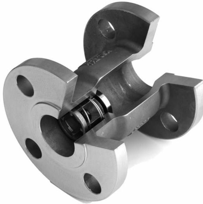
The **Check-All Flanged & Drilled (HV)** check valve is a one piece cast body valve with ASME/ANSI B16.5 Class 150 flanged ends. The HVFD series valve is used when higher flow rates and lower pressure drops are required. The valve is available in sizes 1 inch through 10 inches and standard materials of CF8M (cast 316 stainless), brass and WCB/WCC (cast carbon steel). The HVFD series valve is designed for use with mating ANSI class 150 flanges. Other materials are available upon request.
