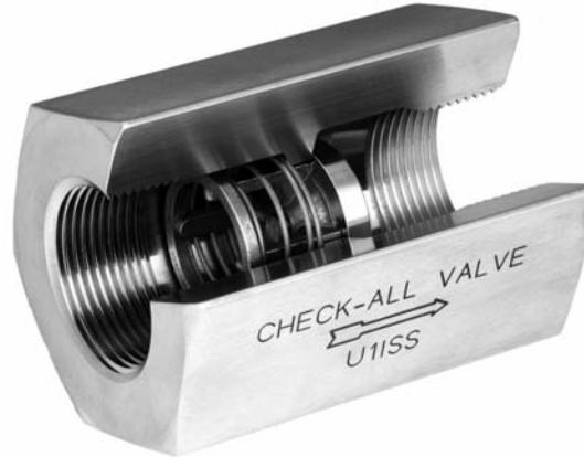
The **Universal High Pressure (U1)** check valve is a one piece body machined from bar stock with female pipe threads. The valve is designed and manufactured for high pressure applications. This valve is normally supplied with a “metal-to-metal” seat. Threads are per ASME B1.20.1. Also available with ISO 7 “Rp” threads. (R1)
