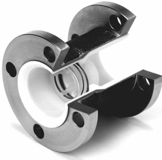
The **Check-All Flanged & Drilled — Fluoropolymer (PTFE) Lined (HT)** check valve is a one piece body with ANSI/ASME B16.5 Class 150 flanged ends. The valve has a solid one piece PTFE liner which covers the flange faces out to the raised face diameter. All wetted surfaces are fluoropolymer (PTFE/FEP/PFA) including the FEP encapsulated stainless steel spring.
