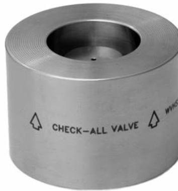
The **Wafer Insert (WV)** valve is designed to fit between two mating ANSI flanges. Two gaskets are required, instead of the one normally used in a flanged joint. The “drop in” valve body fits inside the bolt circle for quick installation and removal in rigid piping applications where the use of the F1, F6, or FP (**see our Flange Insert series on page 6**) is not practical. Many valves in this series meet API 594 requirements. Consult the factory for complete details.
