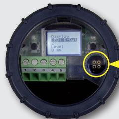
Connection plug for MPI-200-F adapter as an intermediate plug between the ILM-4 electronics and the MPI-200 connection 3 (see next figure).
