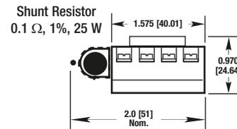
5A 8-Pin Socket with Shunt, 600 V Rating
