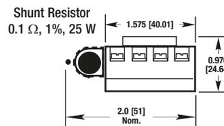
API 6010 G 5A 8-Pin Socket with Shunt, 600 V Rating
