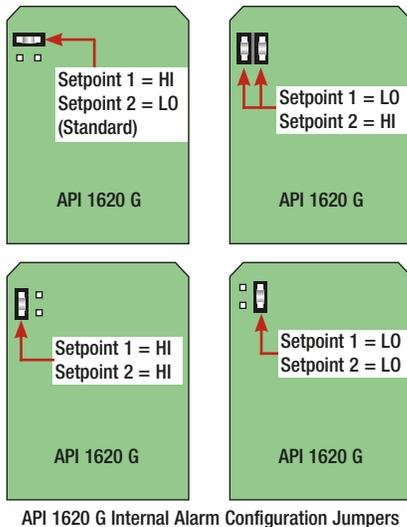
API 1620 G Internal Alarm Configuration Jumpers
