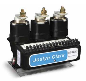
The control module contains the coil and auxiliary contacts wired to a terminal block and is easily removed for checking or immediate replacement. The phase assembly and the control module are the only two replacement parts. The phase assembly is a vacuum interrupter containing the power switching contacts.
