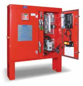
Standard features include green LED for normal power source and red for emergency. Red light and audibly alarm with silence button to monitor the opening of the emergency supply isolation switch. Also, N.O. and N.C. contacts are provided for remote signal of this switch position.
