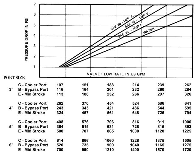
NOTE 1: Cv coefficients coincide with figures in first column.
