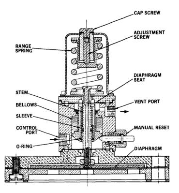
Figure 2 (Control port shown rotated 90° from true position) Models 84378-C1 and 84378-C2 shown
