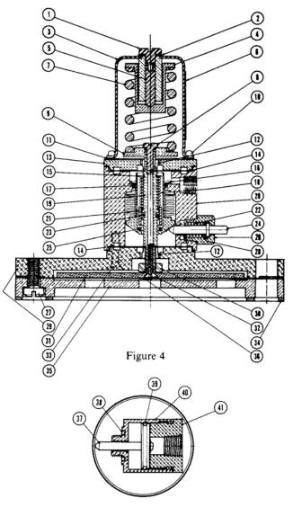
Remote Manual Reset Assembly For 84378-El (85274-Al)
