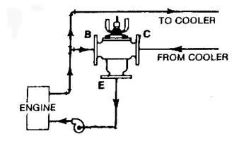
**Figure 4 - Diverting** This figure illustrates a method of controlling the cooling of engine lubricating oil.
