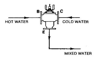
**Figure 2 - Mixing** This figure illustrates a simple means for mixing hot and cold water where a rough mixing is suitable.
