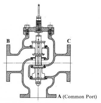
With stem up, port B is open. With stem down, port C is open.
