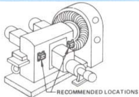
HORIZONTAL OPPOSED RECIPROCATING COMPRESSOR
