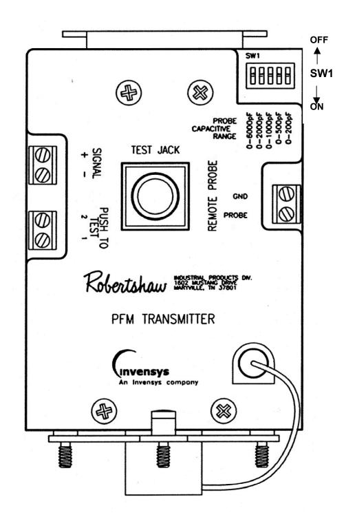
Figure 2.1 Switch SW1 for Selection of Capacitance Range
