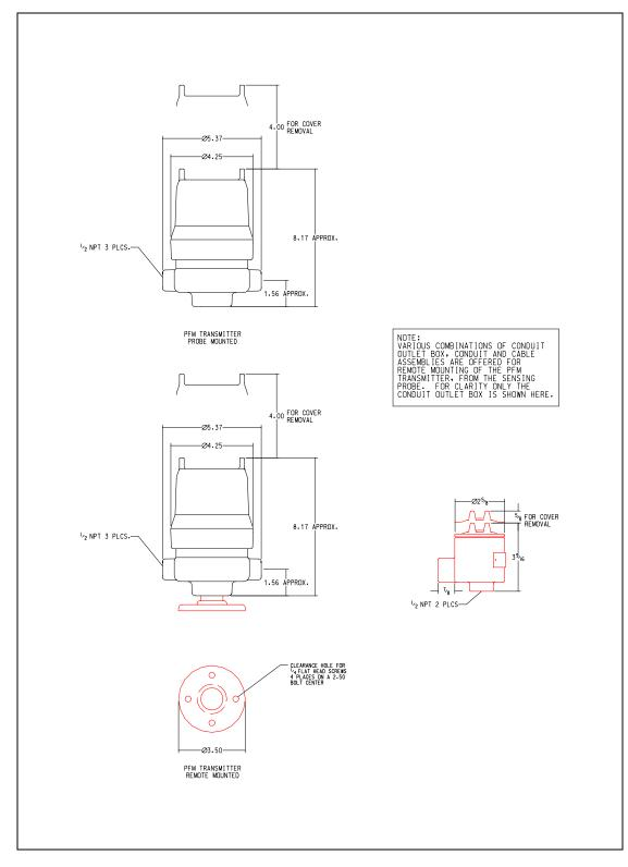
Figure 3.1 Dimensions PFM Transmitter and Probe Mounted Conduit Outlet Box
