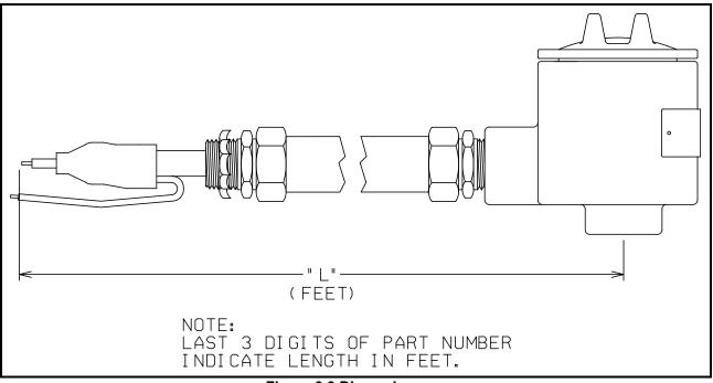
Figure 3.3 Dimensions Conduit Outlet Box, Conduit And Cable Assembly General Purpose, NEMA 4 & NEMA 4X K(032C710-XX, 032KC810-XX & 032KC910-XX)
