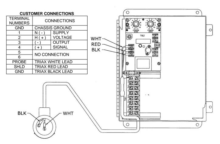
ELECTRICAL CONNECTIONS FOR LARGE WEATHERTIGHT ENCLOSURE (TABLE 3 DESIGNATION E)
