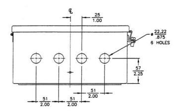
MOUNTING DIMENSIONS FOR 158A LARGE WEATHERTIGHT ENCLOSURE WITH INDICATOR (TABLE 3 DESIGNATION E)
