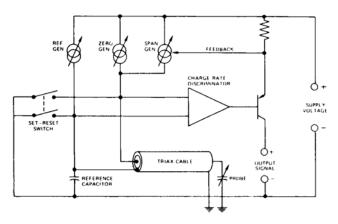
Connected directly across both capacitors is the "charge rate discriminator" amplifier which produces a voltage output when the charging rate of the probe capacitor differs from that of the reference capacitor. When a change in probe capacitance occurs (due to a change in process level), the discriminator amplifier causes an output signal change, which, with voltage feedback, readjusts the probe charging rate through the span generator until the charging rates are again equal.
