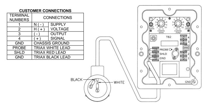
ELECTRICAL CONNECTIONS FOR WEATHERTIGHT AND EXPLOSION PROOF ENCLOSURES (TABLE 3 DESIGNATIONS A, B, C & D)
