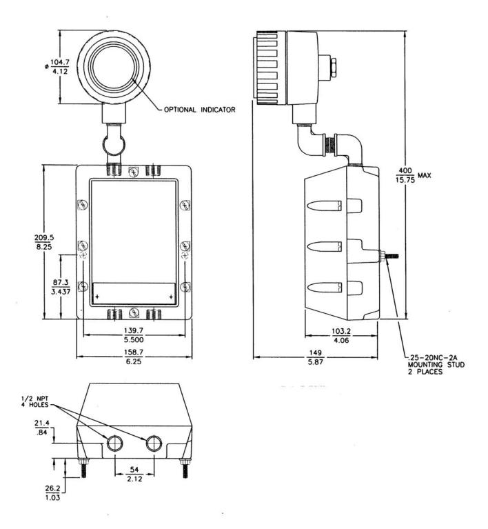
MOUNTING DIMENSIONS FOR 158A EXPLOSION PROOF ENCLOSURE WITH AND WITHOUT INDICATOR (TABLE 3 DESIGNATIONS C & D)
