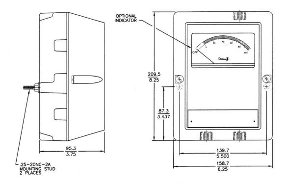
MOUNTING DIMENSIONS FOR 158A WEATHERTIGHT ENCLOSURE WITH AND WITHOUT INDICATOR (TABLE 3 DESIGNATIONS A & B)
