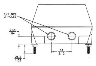
DIMENSIONS OF PROBE MOUNTED CONDUIT
