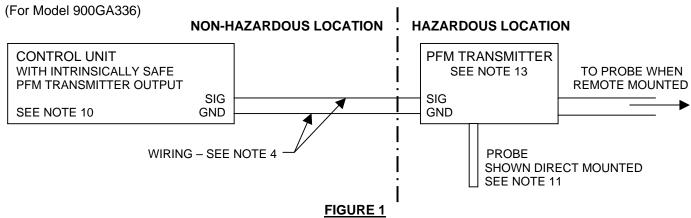
WHEN CONNECTED AS SHOWN THE PFM TRANSMITTER AND PROBE ARE INTRINSICALLY SAFE FOR HAZARDOUS LOCATIONS. SEE NOTE 10
