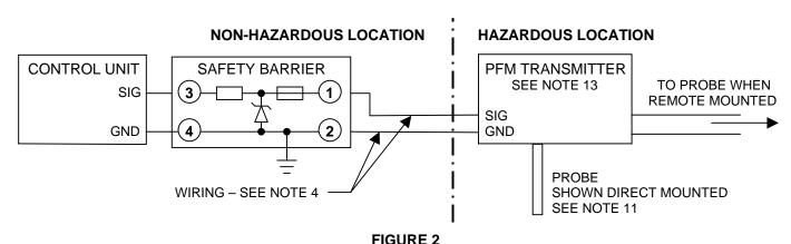
WHEN CONNECTED AS SHOWN THE PFM TRANSMITTER AND PROBE ARE INTRINSICALLY SAFE FOR HAZARDOUS LOCATIONS:
