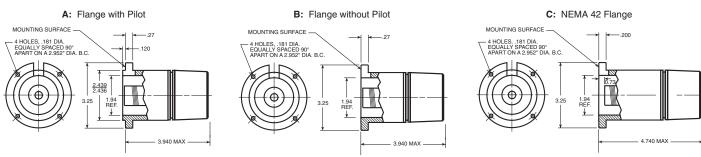
Mating shaft lengths: Typically: 0.5" max. available into the coupling as measured from the A/B mounting surface.
