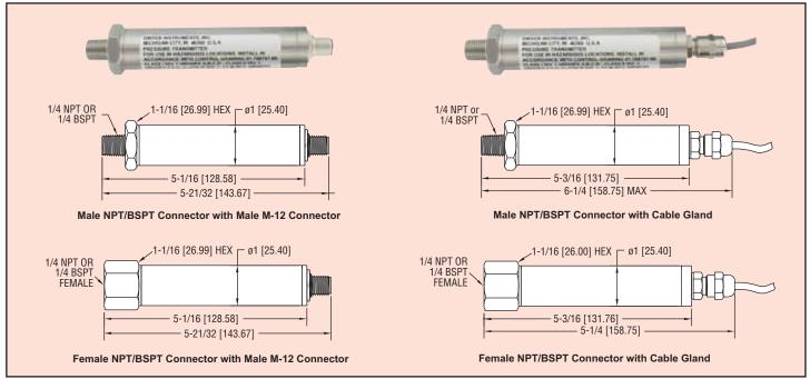
The Series IS626 Intrinsically Safe Pressure Transmitter converts pressure into a standard 4-20 mA output signal. The Series IS626 can be used to accurately measure compatible gases and liquids compatible with its 316/316Lstainless steel wetted parts. Series IS626 full scale accuracy is 0.25%. Designed for industrial environments with a NEMA 4X (IP66) housing, this transmitter resists most effects of shock and vibration. Models are available with a 3' cable or M-12 4 pin connection.
