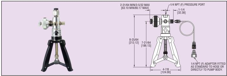
**Verify calibration** of pressure transmitters, switches, controllers, indicators, and recorders with Model PHP Pneumatic Hand Pump. The Model PHP is a hand operated pump for sourcing pressure and vacuum. Use in conjunction with an analog or digital gage for a complete calibration system.
