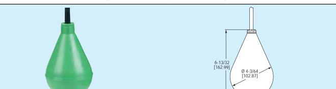
Series FSW Free-Floating Level Switch is a dual level switch designed for filling and draining of tanks, wells, and reservoirs. The shape and interior balance weight ensure impurities and dirt will not adhere to the surface, making it ideal for sewage and waste water applications. The mercury-free switch is designed with an inverter microswitch housed in a polypropylene cover.
