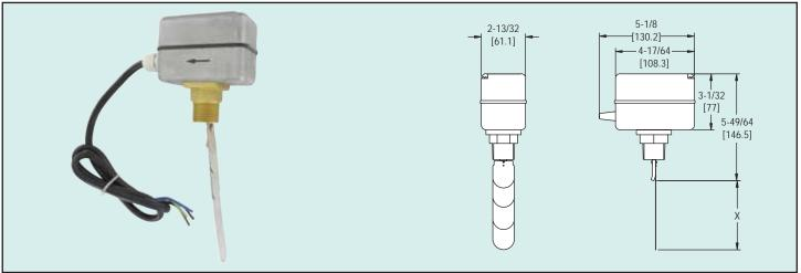
The Model FS-2 Vane Flow Switch offers an economical flow proving solution. Custom set points tailored for the application are enabled by field adjustable vane layers and a set point adjustment screw. The FS-2 features an aluminum weatherproof housing for outdoor installation. Paddles are adjustable to fit 1" to 8" size pipe. FS-2 is ideal for use in "flow or no flow" applications in cold and hot water systems. Perfect for proving flow in boilers, hot water heaters, and chillers.
