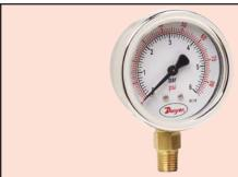
The Series 63000M Liquid Filled Pressure Gages provide superior performance in applications where vibration, pulsation, mechanical shock and pressure spikes are common. The Series 63000M gages have dual English/metric scales with ±1.6% full scale accuracy and are available in 2.5" dial sizes. Units are designed with 304 SS housings and brass wetted parts. These gages can withstand ambient temperatures up to 140°F (60°C) and process temperatures
