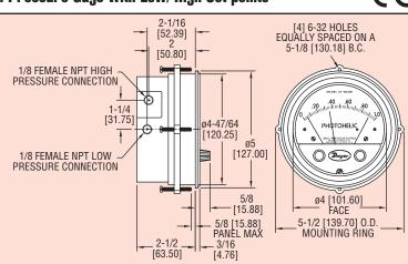
Using solid state technology, the Series 3000MR and 3000MRS Photohelic® switch/gages combine the functions of a precise, highly repeatable differential pressure
