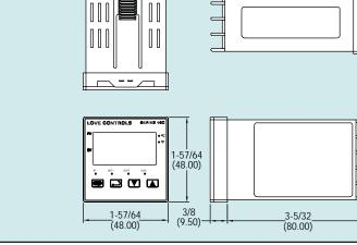
**The compact Series 16C Temperature Controller** offers accurate temperature measurement and control in a 1/16 DIN package. Designed for direct or reverse acting (cooling or heating) control, the Series 16C can be programmed for simple ON/OFF or more complex PID control functions. PID control is supported with manual or autotuning. Select relay, voltage or current output for control methods.
