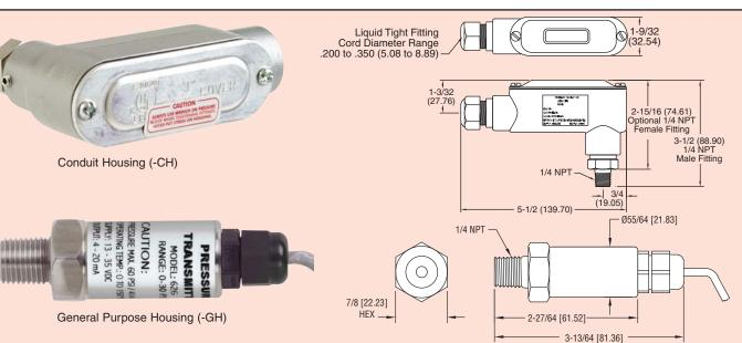
**The Dwyer Series 626 Pressure Transmitters** possess a highly precise 0.25% piezo-resistive sensor contained in a compact, rugged, NEMA 4X stainless steel general purpose housing or cast aluminum conduit housing.
