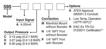
\*ATEX Exd, FM/CSA Explosionproof, EAC EX -40°F to 158°F (-40°C to 70°C) operation only \*\*R option must be combined with K option
