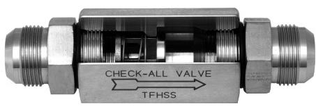
The Tubing Check Valve-Flared (TF) is a three-piece constructed check valve with 37° flared end fittings that conform to SAE J514 & ISO 8434-2. These valves are designed for maximum flow with minimal pressure drop. Consult the factory for more information.
