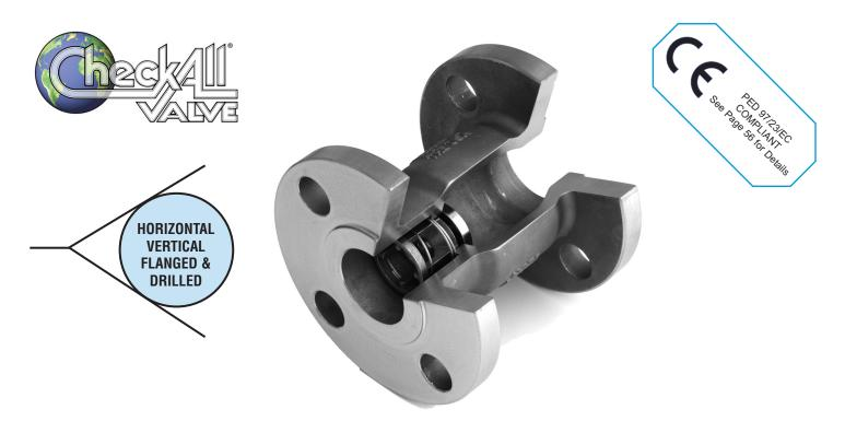
The **Check-All Flanged & Drilled (HV)** check valve is a one piece cast body valve with ASME/ANSI B16.5 Class 150 flanged ends. The HVFD series valve is used when higher flow rates and lower pressure drops are required. The valve is available in sizes 1 inch through 10 inches and standard materials of CF8M (cast 316 stainless), brass and WCB/WCC (cast carbon steel). The HVFD series valve is designed for use with mating ANSI class 150 flanges. Other materials are available upon request.
