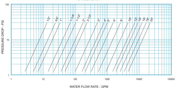
**Note:** All flow curves and Cv values presume the valves are fully open with 1/2 PSI cracking pressure springs. Consult the factory for more information.
