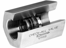
The **Universal High Pressure (U1)** check valve is a one piece body machined from bar stock with female pipe threads. The valve is designed and manufactured for high pressure applications. This valve is normally supplied with a "metal-to-metal" seat. Threads are per ASME B1.20.1. Also available with ISO 7 "Rp" threads. (R1)
