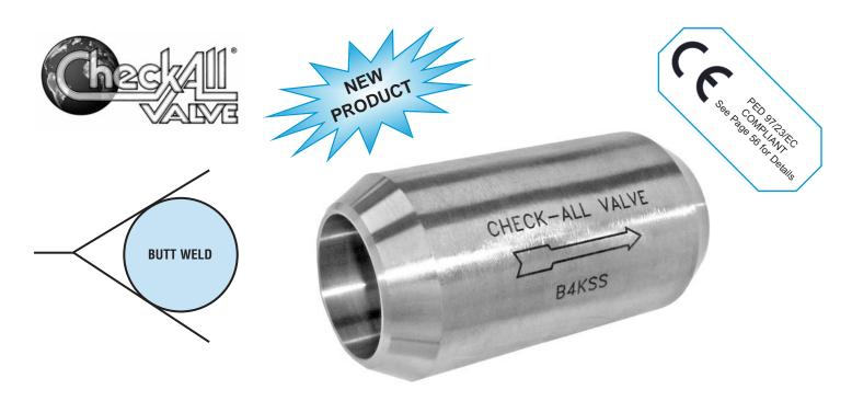
The **Butt Weld (B4)** check valve is a one piece body machined from bar stock, eliminating porosity concerns and providing uniform density for more consistent welds. Made to ASME/ANSI B16.25 for schedule 40 pipe, it carries rugged, dependable Check-All trim with a wide variety of seat materials and cracking pressures to choose from. This makes the **Butt Weld** valve the obvious choice.
