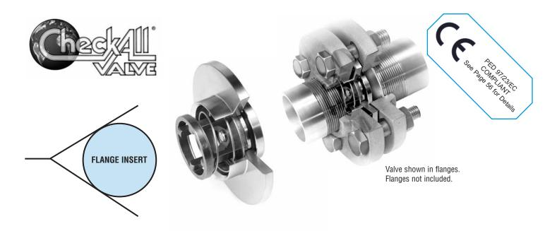
The **Flange Insert (F1, F6, FP)** valves are the ultimate check valves in flanged systems. They provide the simplest and most economical way to install check valves in a piping system. The valve body helps position itself while bolts are being installed and tightened. Two gaskets are required instead of the one normally used in a flanged joint. See page 52 or consult the factory for additional installation guidelines.
