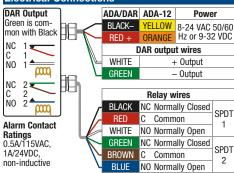
The ADA 2-conductor cable or the DAR 4-conductor cable with the RED and BLACK leads is for the gauge power supply. ADA models with the 12 foot lead option use an 8 conductor cable with YELLOW and ORANGE power leads.
