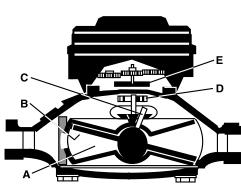
Liquid flowing through the meter chamber (A) causes a disc (B) to nutate or wobble. This motion, in turn, results in the rotation of a spindle (C) and drive magnet (D). Rotation is transmitted through the wall of the meter to a second magnet (E) or varied style of sensor pickup.
