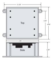
Figure 3: Plastic enclosure dimensions
