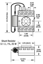
API 6010 G 5A 8-Pin Socket with Shunt, 600 V Rating
