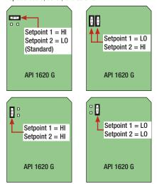
API 1620 G Internal Alarm Configuration Jumpers
