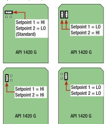
API 1420 G Internal Alarm Configuration Jumpers
